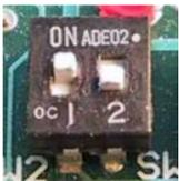
To enable this mode of operation position the **dip switch 1 on ON**
